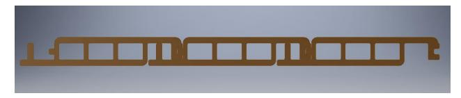
In the above image, the boards were installed starting at the right side and moving left. This installation will require **RIGHT END CAPS**.
