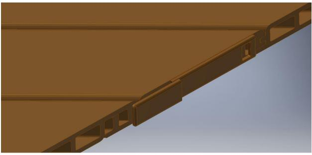
6. Cut the second end cap and insert it into the end of the DuxxBak board. Use LEXEL brand adhesive or silicone to better secure the end cap if necessary. When done properly, only a small seam will be visible where the two end caps meet.
